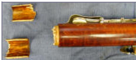
Woodwind Bassoon Tenon Repair Before Repair
