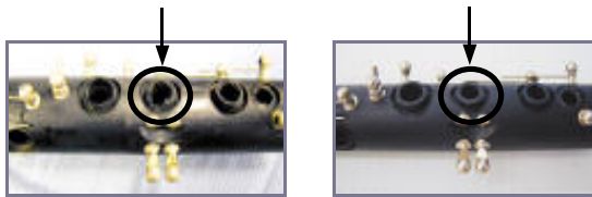
Woodwind Tone Hole Repair Before & After
